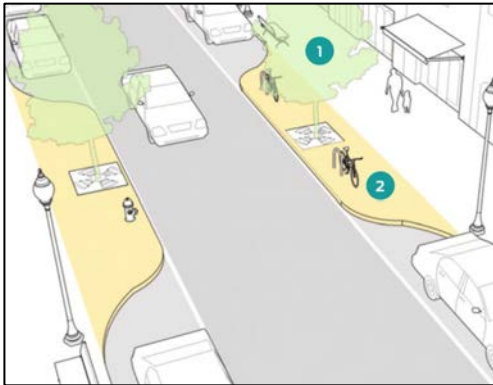
Pinch Points, which are used at midblock narrow roads, narrow roads and increase public pedestrian space.
