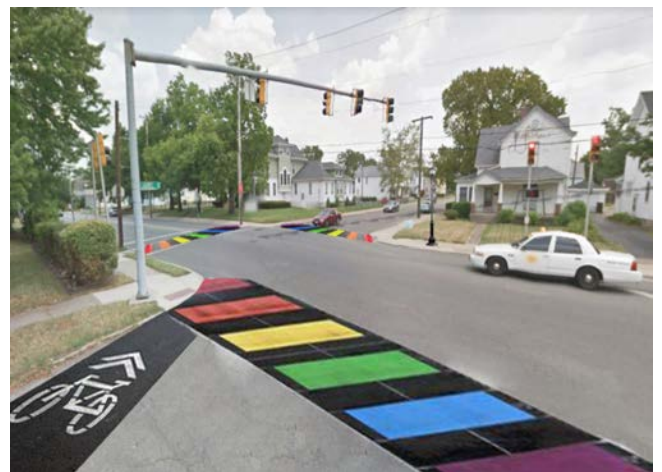
Recommended bike lane on Laurel Avenue and colored crosswalk to alert drivers of pedestrian activity
