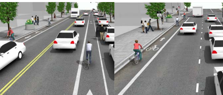
Left-Side Bike Lane for use on one-way streets, NACTO Guide Conventional bike lane, an exclusive space for bicyclists, NACTO Guide
